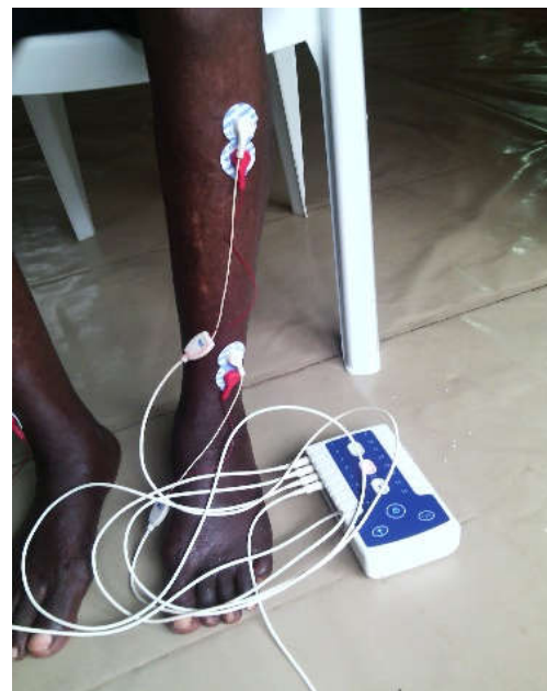
Recording of EMG signals by the WiFi modem and the computer
