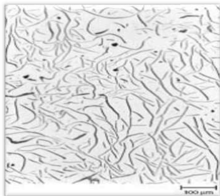
a) Grey cast iron with lamellar graphite
