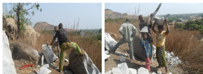
Photo a: Fragmentation of stone blocks by men Photo b: Loading of stone blocks by women
