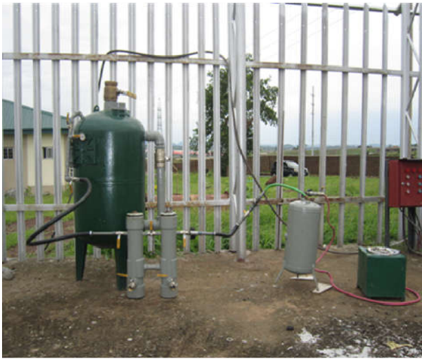
Figure 1. 150 Litres Anaerobic Biodigester, designed and constructed by Hilili Johnson & Dandy Onurah (2013)
