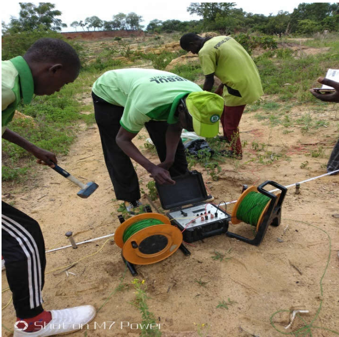
Figure 4. Field Survey using Omega Resistivity Meter in Schulumberger Electrode Configuration
