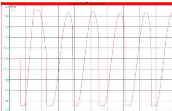
Fig. 6. Simulation result of the DC-AC Converter stage without filtering
