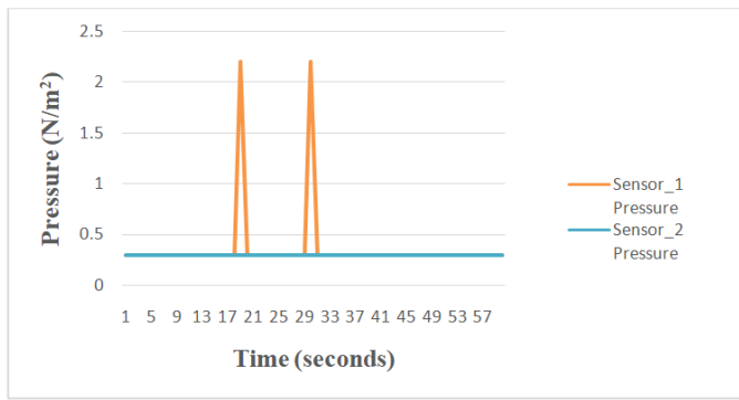
Figure 14. Pressure Values for Sensor_1 and Sensor_2 for no Flow and no Leakage Case (Vertical Configuration)
