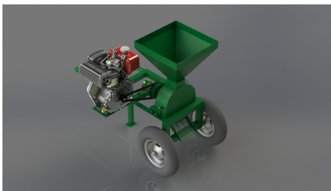
Figure 8. Three dimensional model of the developed palm kernel nut cracking machine
