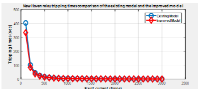
Figure 6. New Haven relay tripping times comparison of the existing model and the improved model
