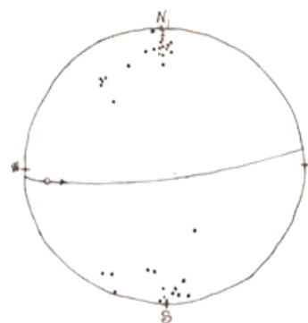
Figure 4. Determination of Syncline 1 from So stratification planes on Wulff stereographic canvas
