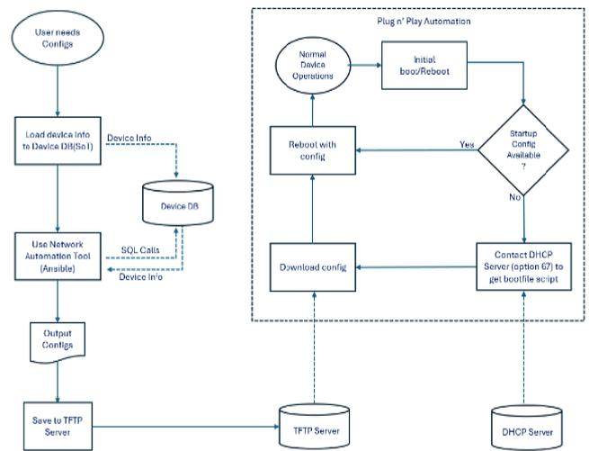
Figure 7. Zero-Based Provisioning (ZTP) Workflow
