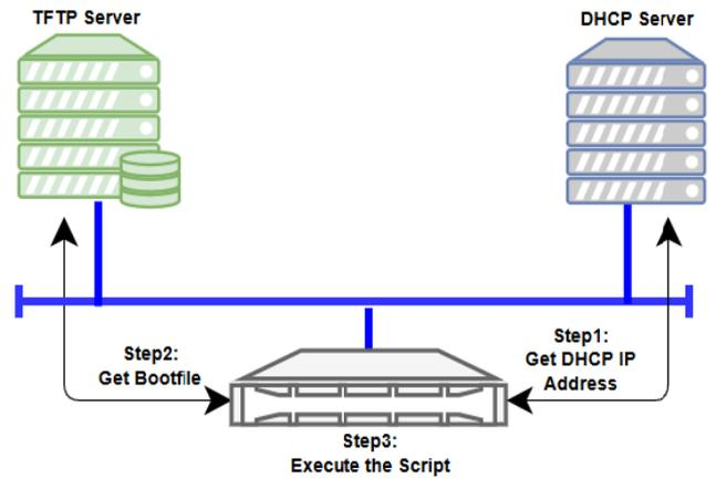
Figure 6. Zero-Based Provisioning Processes
