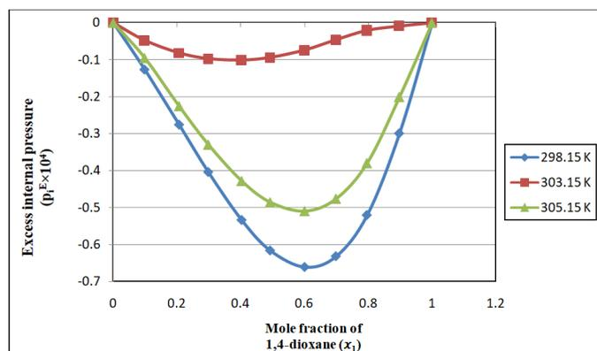
Figure 5. Curves of excess internal pressure ( $P_i^E$ ) against the mole fraction of 1,4-dioxane  $x_1$ , for the binary mixture (1,4-dioxane (1) + 1-Octanol (2)) at different temperatures (blue  $\diamond$ , 298.15 K orange  $\blacksquare$ , 303.15 K and gray  $\blacktriangle$ , 305.15 K). The solid lines represent the values calculated from the Redlich–Kister equation
