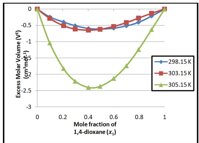
Figure 1. Curves of excess molar volume  $V^E$  against the mole fraction of 1, 4-dioxane  $x_1$ , for the binary mixture (1,4-dioxane (1) + 1-Octanol (2)) at different temperatures (blue  $\diamond$ , 298.15 K orange  $\blacksquare$ , 303.15 K and gray  $\blacktriangle$ , 305.15 K). The solid lines represent the values calculated from the Redlich–Kister equation
