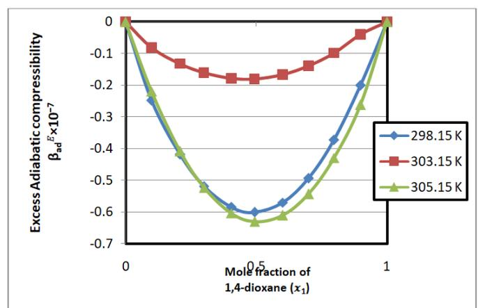
Figure 2. Curves of excess adiabatic compressibility  $\beta_{ad}^E$  against the mole fraction of 1,4-dioxane  $x_1$ , for the binary mixture (1,4-dioxane (1) + 1-Octanol (2)) at different temperatures (blue  $\diamond$ , 298.15 K orange  $\blacksquare$ , 303.15 K and gray  $\blacktriangle$ , 305.15 K). The solid lines represent the values calculated from the Redlich–Kister equation.
