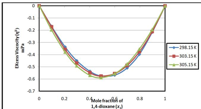
Figure 3. Curves of excess viscosity  $\eta^E$  against the mole fraction of 1,4-dioxane  $x_1$ , for the binary mixture (1,4-dioxane (1) + 1-Octanol (2)) at different temperatures (blue  $\diamond$ , 298.15 K orange  $\blacksquare$ , 303.15 K and gray  $\blacktriangle$ , 305.15 K). The solid lines represent the values calculated from the Redlich–Kister equation
